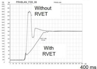
In this example, a vented anti-shock relief valve RV\*T is used in a bypass leg of a pressure reducing valve. Port 3 of the RV\*T is plugged. In the set up for the test, the 2/2-way directional valve represents a cylinder that either moves freely or stops. In the example, a direct-acting PR\*B controls the pressure. The RV\*T controls the rate of pressure rise only and not the final controlled pressure level.
