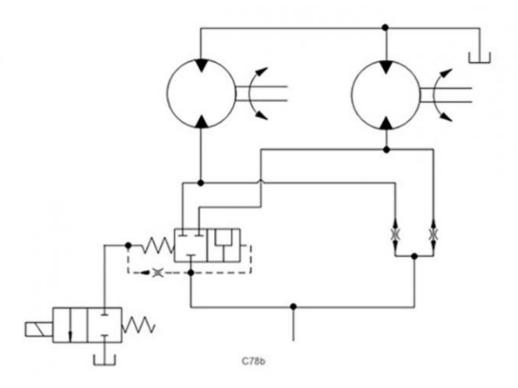
The example shows a 2/3-way directional valve that is commonly used in parallel with a flow divider.
