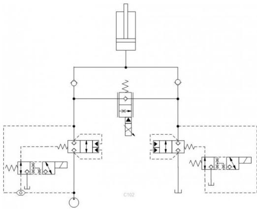
The example shows a proportional valve and logic elements in a circuit for lifting and lowering a single-acting cylinder
