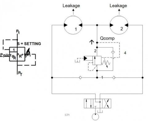
In this circuit, two motors in series are mechanically connected (not shown). Since motors have internal leakage, the motor downstream would tend to rotate slower and will then be driven by the external mechanical force. As a result, the first motor exerts a higher torque than the second motor and there is a loss in efficiency.
