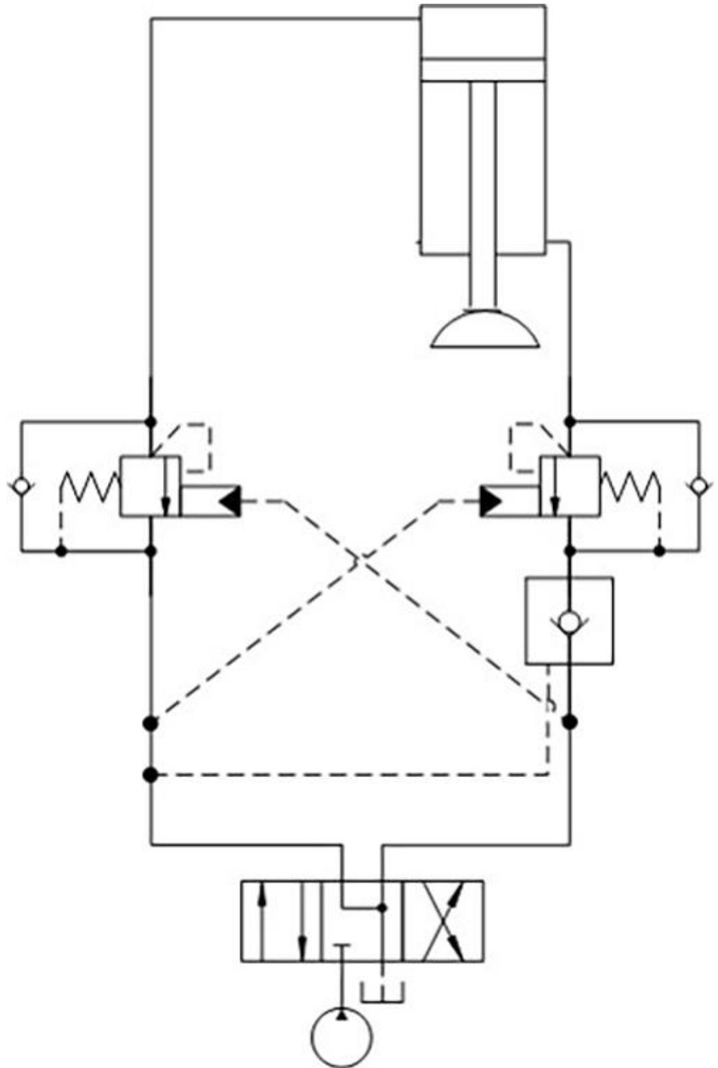
The circuit shows a counterbalance valve CB in series with a standard pilot-to-open check valve CK on the cylinder rod end and a second counterbalance valve on the full bore end of the cylinder.
