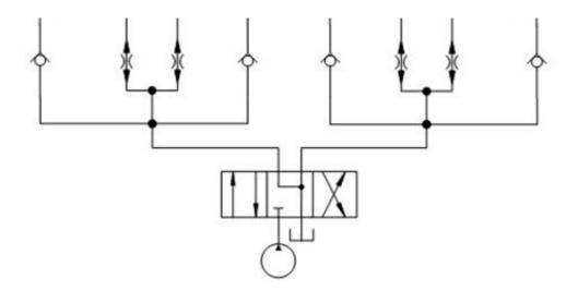
This example shows flow dividers with reverse free-flow check valves and cylinders with counterbalance valves.
