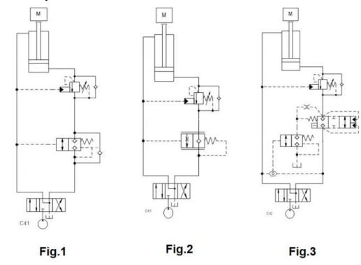
The circuits show three examples for redundancy in load-holding applications with counterbalance valves using balanced logic valves.
