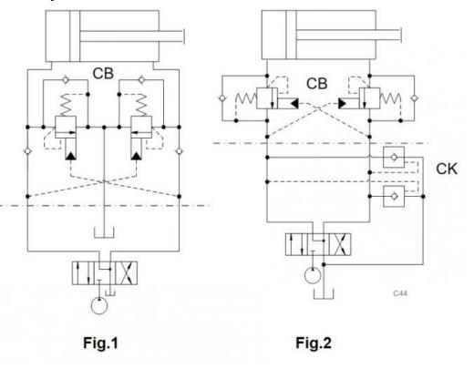
The example shows two circuits that deal with pressure in the return line of counterbalance valves.
